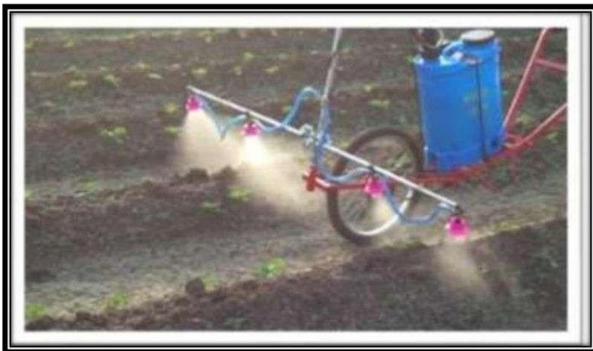
Fig 1.1(a) mechanical multi nozzle wheel sprayer
