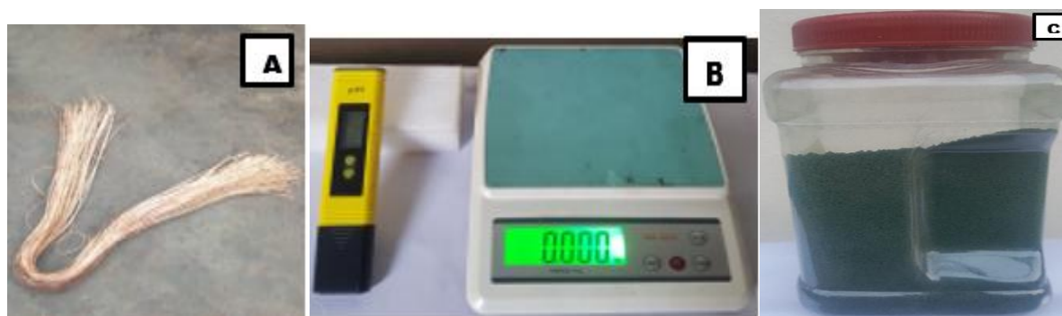
Figure 2.1: Extracted Raffia palm fibre (a) Digital weighing balance and pH used (b) Phenolic Resin used (c)
