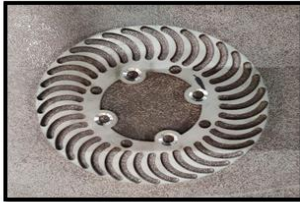
Fig. 3.1.2.1. Rotor made out of SS420
