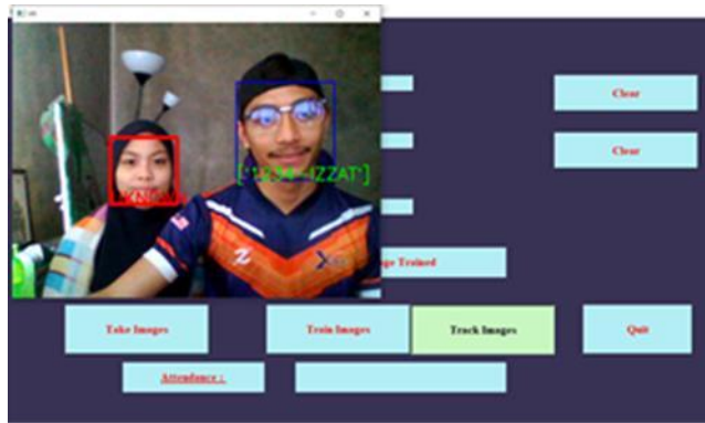
Figure. 8 : The system will detect the check in passenger as name shown on the screen in greencolour and the red colour shown as unknown person
